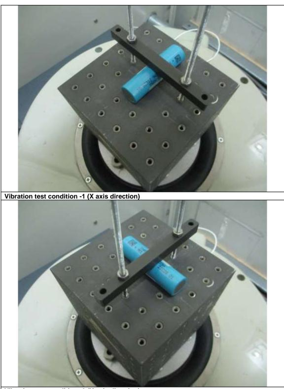
Vibration test condition -2 (Y axis direction)
