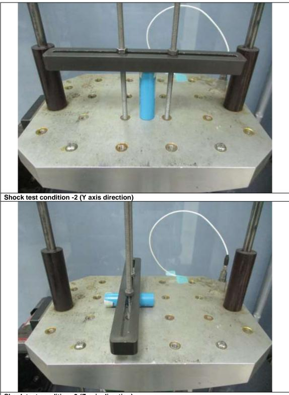
Shock test condition -3 (Z axis direction)
