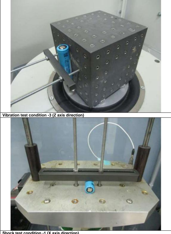
Shock test condition -1 (X axis direction)
